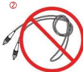
3. Never use the fiber to pick up or drag the device to which it is attached. Doing so may break the optical fiber inside the item. (See fig.3)
