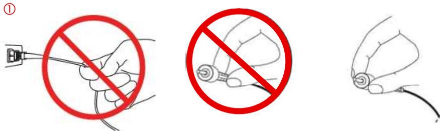
2. Do not allow kinks or knots to develop in the fiber. Do not pull the fiber when kinks or knots are present. Carefully work out any tangles. Knots, kinks, twists and bends in the optical fiber will ruin the fiber's ability to transmit light. When bending the optical fiber product, do not bend it excessively. Doing so may break the optical fiber inside the product. In many cases, a bend or break in an optical fiber will completely disrupt the system's performance. (See fig.2)
